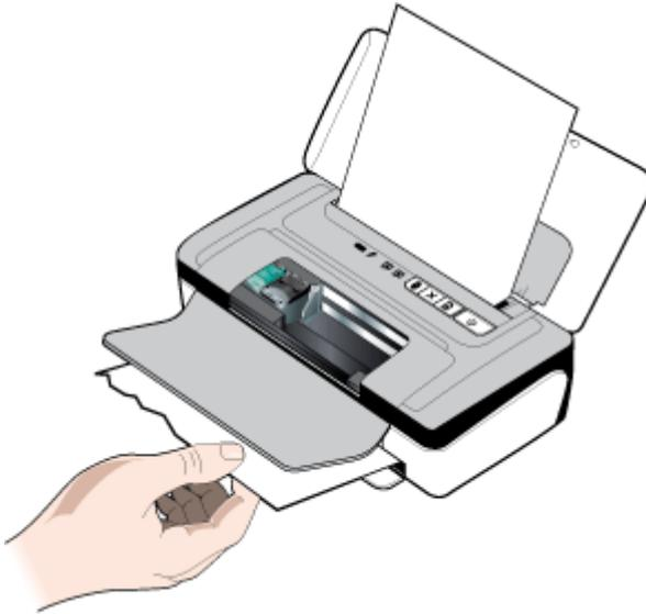
7. If the jammed media is not visible in the print area inside the printer, remove what is visible in the input tray.
