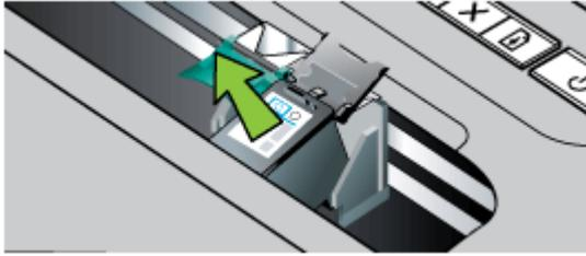
4. Insert the new ink cartridge into its cradle compartment at the same angle at which you removed the old ink cartridge. Check the symbol on the latch against the symbol on the ink cartridge to make sure you are inserting the correct ink cartridge.
