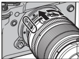
**!** When attaching lenses, ensure that dust or other foreign matter does not enter the camera and be careful not to touch the camera's internal parts. Do not press the lens release button while attaching the lens and be sure the latch has securely clicked into place.
