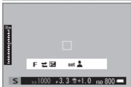
**📄** The front command dial can be used to set exposure compensation to values between  $-5$  and  $+5$  EV.
