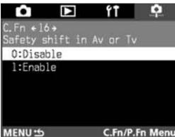
Safety shift can be set for the shutter-priority AE and aperture-priority AE modes.
