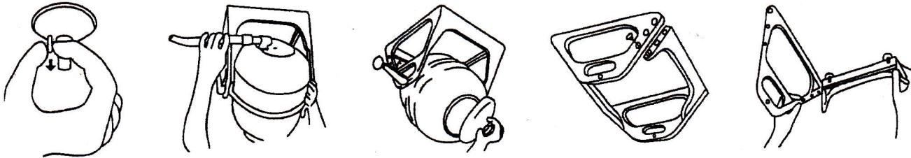
The suction cups are designed to hold the machine in place during washing. There are small tabs in the front part of the suction cups, which are specially designed for removing the machine. You pull up on these tabs to easily remove the suction cup from the surface, if necessary (the suction force will vary depending upon the surface).
