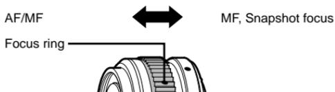
With snapshot focus, a distance is set using the focus ring based on the shooting distance. The camera focuses over a depth of field corresponding to the set aperture value.
