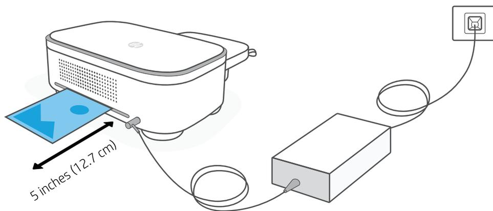
When the photo prints from the HP Sprocket printer, it passes through the printer and emerges multiple times. The picture gets colors applied to the photo with each iteration.
