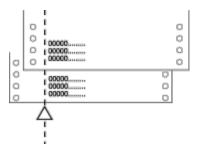
For single sheets, printing starts at "0" on the paper guide scale. The unprintable area is to the left of the "0."
