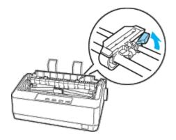
Slide the left sprocket using the arrow mark on the printer as a guide. The printer prints to the right of the arrow mark. Push the sprocket lock lever back to lock it in place. Then slide the right sprocket unit to match the width of your paper, but do not lock it. Move the paper support so it is midway between the sprocket units.
