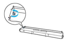
Insert the ribbon cartridge into the printer as shown; then press both sides of the cartridge firmly to fit the plastic hooks into the printer slots.
