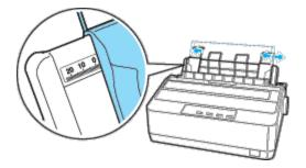
Slide a sheet of paper down firmly between the edge guides until it meets resistance.
