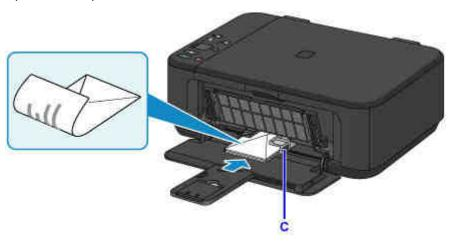
5. Slide the right paper guide (C) to align the paper guides with both sides of the envelopes.
