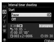
Pictures can be played back and shooting and menu settings can be adjusted freely while interval timer photography is in progress. The monitor will turn off automatically about four seconds before each interval.
