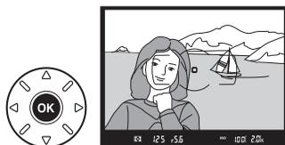
The focus selector lock can be rotated to the locked (L) position following selection to prevent the selected focus point from changing when the multi selector is pressed.
