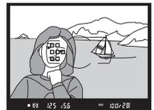
AF-area mode can be selected by pressing the AF-mode button and rotating the sub-command dial until the desired setting is displayed in the viewfinder or control panel.
