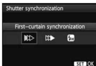
Normally, set this to **[First-curtain synchronization]** so that the flash fires immediately after the exposure starts.
