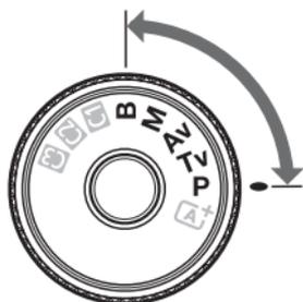
In the **P/Tv/Av/M/B** shooting modes, you can select the shutter speed, aperture, and other camera settings to change the exposure and obtain the desired result.
