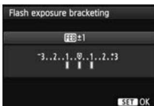
While the flash output is changed automatically, three shots are taken. For details on FEB (Flash Exposure Bracketing), refer to the Speedlite’s instruction manual.
