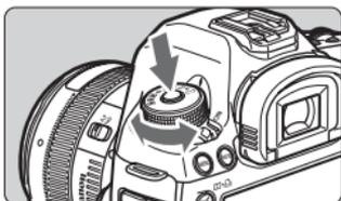
Turn the dial while holding down the lock release button at the center of the dial.
