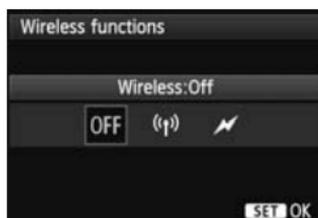
Wireless (multiple) flash shooting is possible with radio or optical transmission. For details on wireless flash, refer to the Speedlite's instruction manual.
