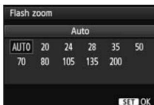
With Speedlites having a zooming flash head, you can set the flash coverage. Normally, set this to **[AUTO]** so that the camera will automatically set the flash coverage to match the lens focal length.
