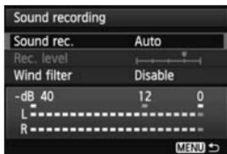
You can shoot movies while recording sound with the built-in monaural microphone or a commercially-available stereo microphone. You can also freely adjust the sound-recording level. Set the sound recording with [**4**: **Sound recording**]. In the <[A+]> mode, this setting is displayed in [**2**].
