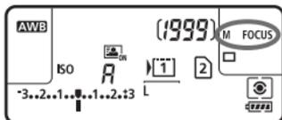
**1** Set the lens focus mode switch to **<MF>**.
