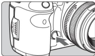
Press the depth-of-field preview button to stop down the lens to the current aperture setting and check the depth of field (range of acceptable focus).
