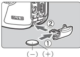
**4 Replace the battery in the battery holder.**
