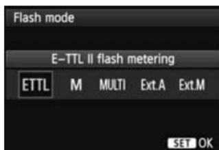
**[E-TTL II flash metering]** is the standard mode of EX-series Speedlites for automatic flash shooting.
