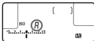
If the ISO speed is set to “A” (Auto), the actual ISO speed to be set will be displayed when you press the shutter button halfway. As indicated below, the ISO speed will be set automatically to suit the shooting mode.
