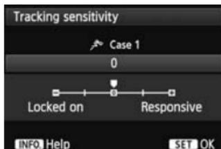
Sets the subject-tracking sensitivity during AI Servo AF when an obstacle enters the AF points or when the AF points stray from the subject.
