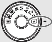
**While holding down the center of the Mode Dial, set it to  $\langle \text{AI}^+ \rangle$  (Scene Intelligent Auto) (p.64).**
