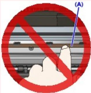
If you soil or scratch the clear film by touching it with paper or your hand, it could damage the machine.
